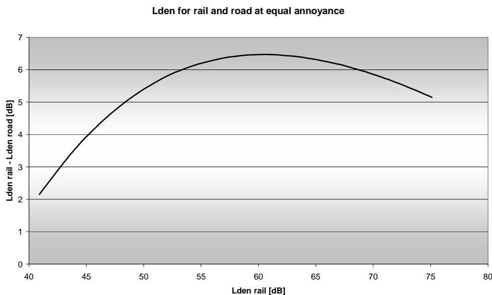
Figure 9: Difference between road traffic noise level and rail traffic noise level (in other words: NACF) at equal percentages of annoyance, derived from Miedema exposure response relationships.
