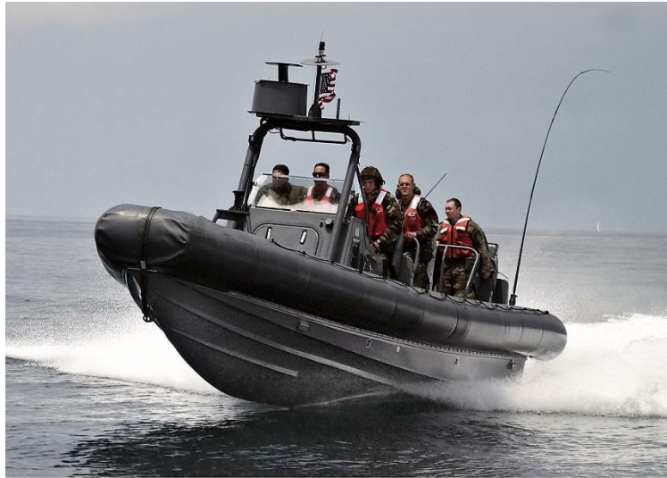
Abbildung 1: Frontansicht eines RHIB der US Navy. Der typische V-förmige Rumpf ist gut zu erkennen. Quelle: US Navy by Photographer's Mate 3rd Class John DeCoursey - This Image was released by the United States Navy with the ID 030922-N-8209D-011.
